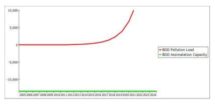
Figure 13. BOD pollution load and BOD assimilation capacity
